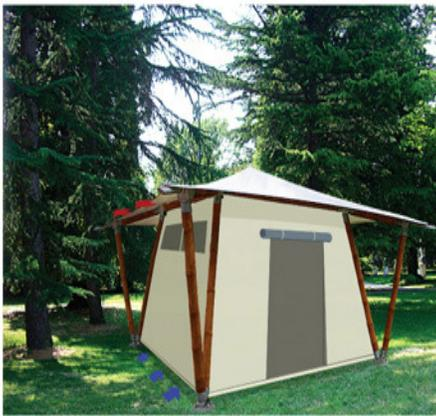
The Natura tent follows the minimalist style of the Bedouin encampments, with the essential weight-bearing frame made of Bamboo cane. It is equipped with steel connections and perimetral closures made of PVC coated fabrics or gore-tex treated fabric. The hardwood platform, with ventilation windows and the suspended ceiling made of micro-perforated material, together activate a passive circulation of air.
